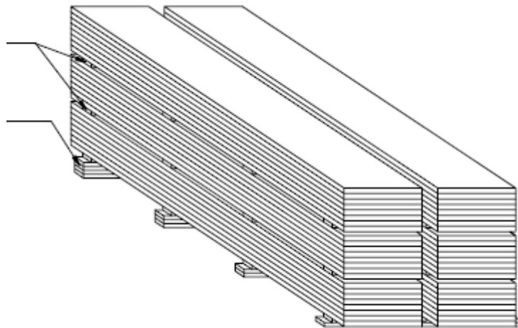
panels . The packages have to be places in dry and ventilated places in order to avoid that on panels or on single sheets placed internally into the packages , phenomena of water stagnation or condense could occur. These phenomena are particularly aggressive on metal sheets with consequent possible formation of white oxidation on the galvanized support..
